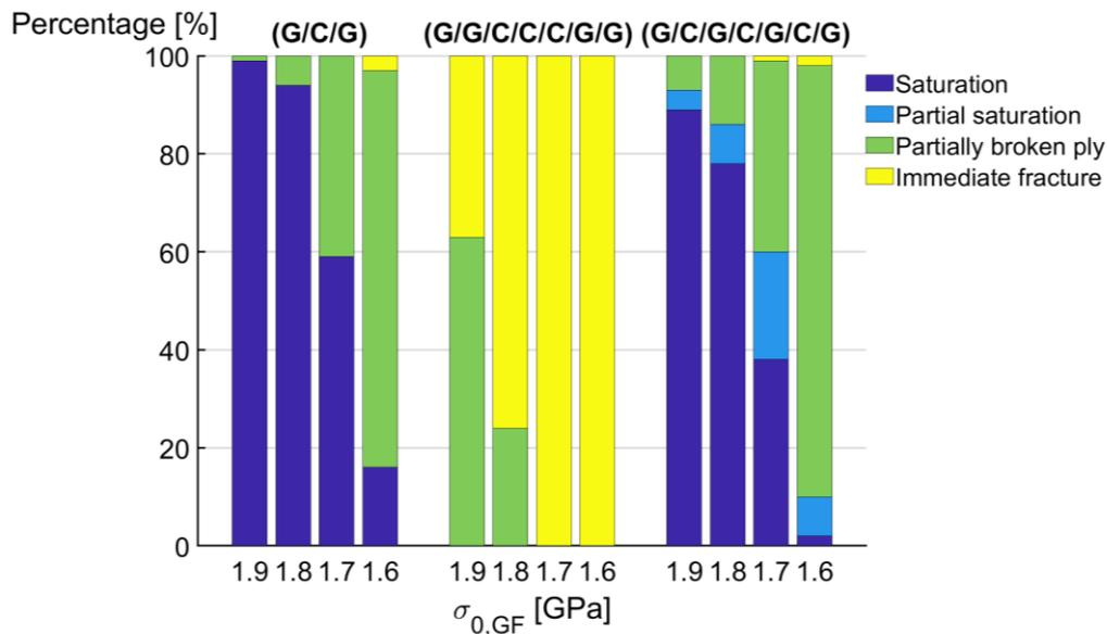
**Figure 4** – Failure mode variation with the  $\sigma_{0,GF}$  for the different stacking sequences tested – fine variation.
