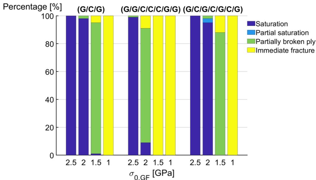
**Figure 3** – Failure mode variation with  $\sigma_{0,GF}$  for the different stacking sequences tested – coarse variation.
