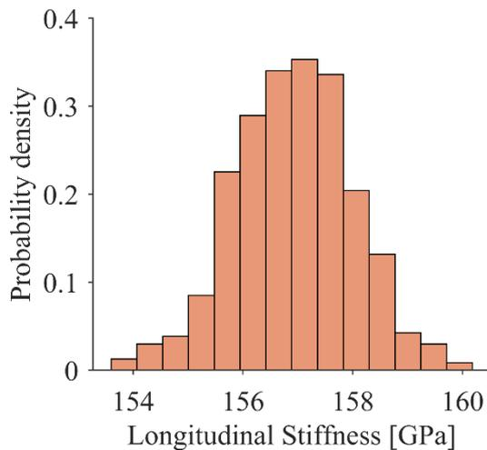
**Figure 7** Probability distribution of longitudinal stiffness obtained with the ply model.
