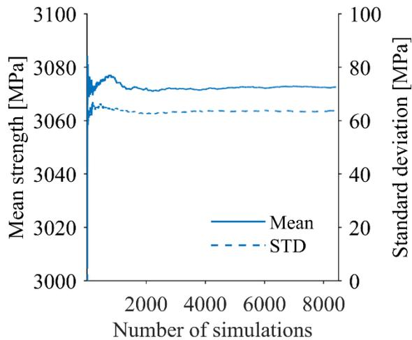
**Figure 4** Convergence of the mean and standard deviation of fibre break model results for  $V_f = 0.5$ .
