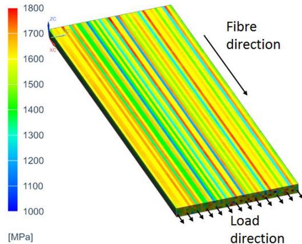
**Figure 2** Longitudinal stress results of the ply model for a virtual coupon. The higher local stresses correspond to higher  $V_f$ .
