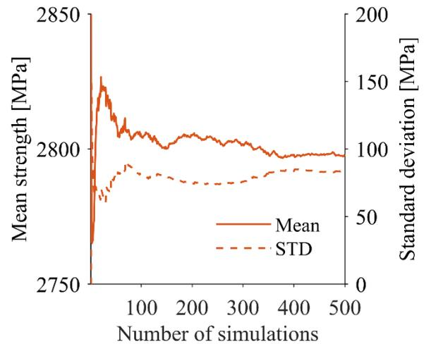
**Figure 3** Convergence of the mean and standard deviation of virtual testing results with the ply model.
