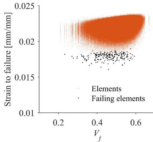
**Figure 6** Strain to failure and  $V_f$  map. Each point represents a single finite element. In black only the failing elements for each coupon are represented.
