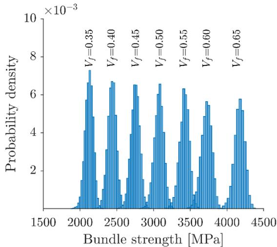
**Figure 1** Probability distributions of bundle strengths for different  $V_f$  calculated with the fibre break model.
