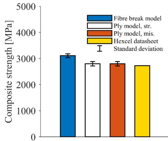
**Figure 8** Comparison between the results obtained with the fibre break model, the ply model with straight fibres, with misalignment and the strength from the datasheet [17].
