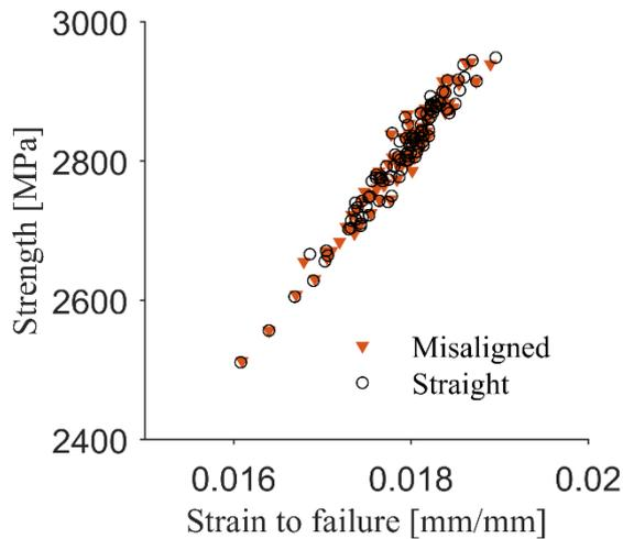
**Figure 5** Failure stress and strain of 100 virtual coupons with and without misalignment.
